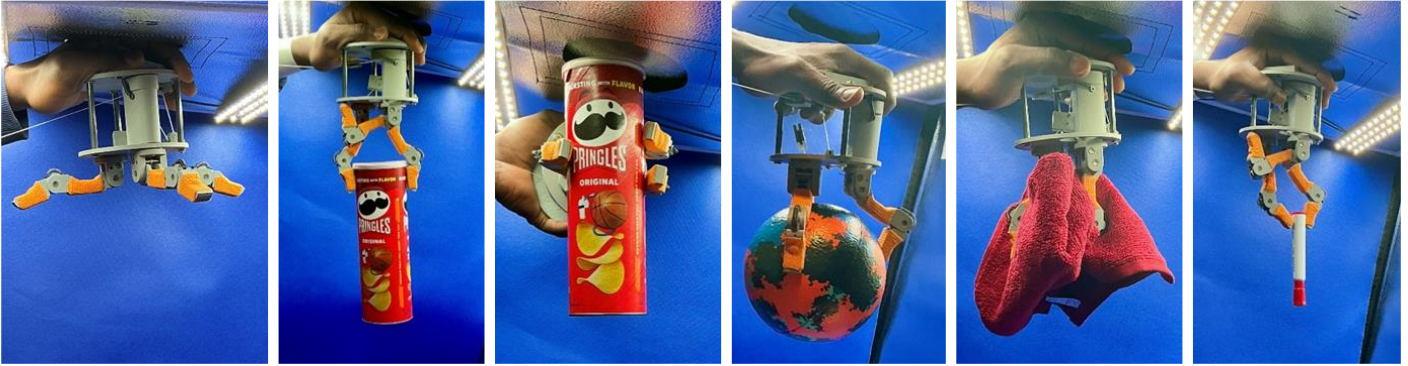
Figure 6. Grasping different objects using the PhaseHand . Left to right: fully open hand configuration, Pringles can is grasped using pinch grasp, Pringles can is grasped using tripod (cylindrical) grasp, soft ball, towel, and marker.
